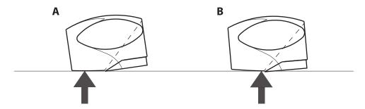
Begin by taking as light of a cut as you can until you get a feel for the "action". Exit a cut by rolling forward onto the toe away from the blade. The natural tendency is to roll backward to exit a cut, however, this will cause the blade to dig in and take a heavy cut.
